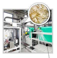
Reliable separation: cavity-specific feedback on the quality of the part.
